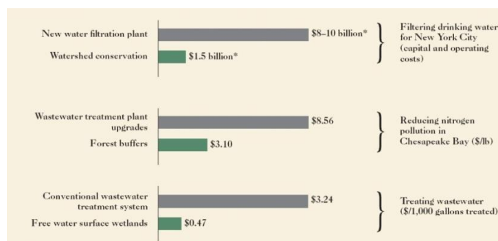
Fig.3. Green Infrastructure Can Be Less Expensive Than Gray Infrastructure Source: Kenny, 2006
